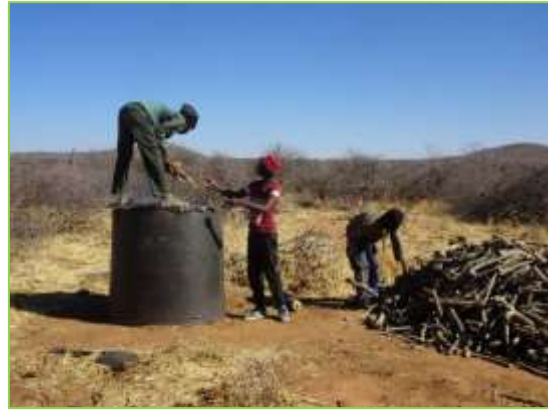
Picture 56: progressively the kiln is filled with wood on top of the fire
