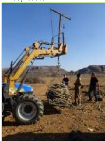
Picture 82: Wood load weighing for one traditional kiln at producer 1
