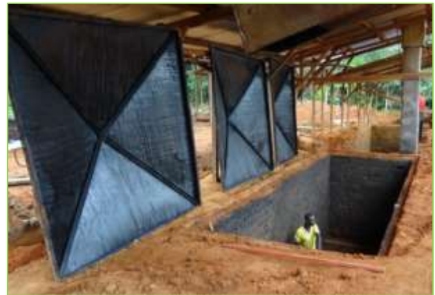
Picture 24: Mindourou Kiln – metal lids
