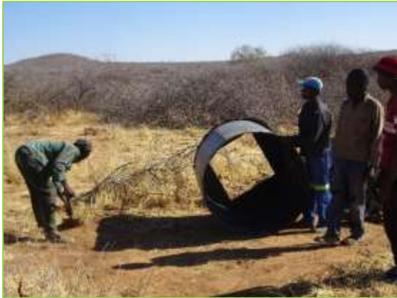
Picture 52: surface cleaning before kiln placement
