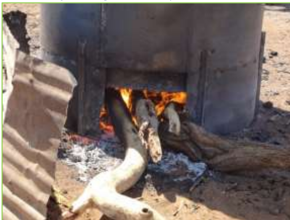
Picture 68: the wood contained in the retort is heated
