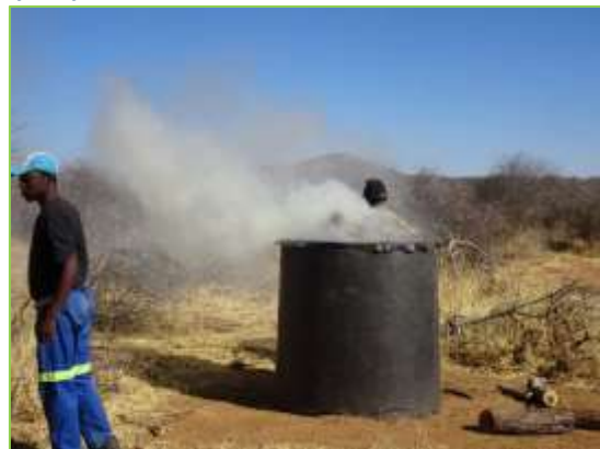
Picture 57: progressively the kiln is filled with wood on top of the fire
