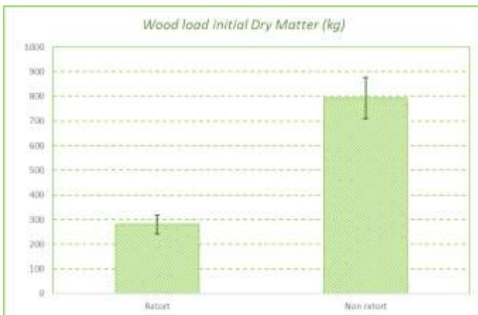
Figure 9: comparison between retort & non retort kilns regarding dry matter wood load
