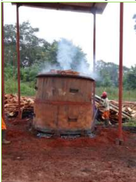
Picture 9: Metal drum (TPI) in Cameroon
