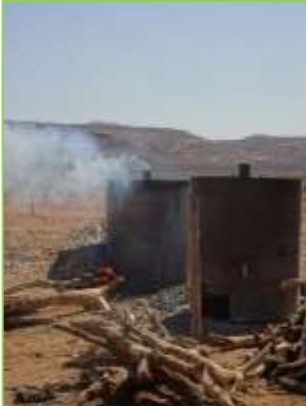
Picture 85: Retort Kiln testing
