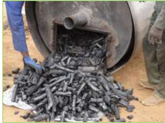
Picture 77: 120 kg charcoal has been produced in 24 h
