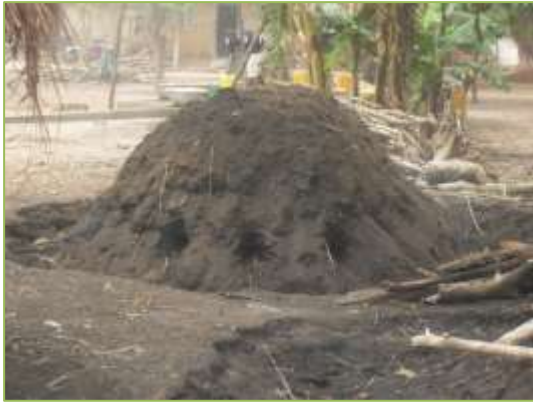
Picture 3: Traditional mound kiln in Benin (wood cut in the forest)
