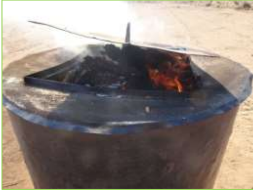
Picture 59: when no wood can be added, the kiln is ready to be sealed
