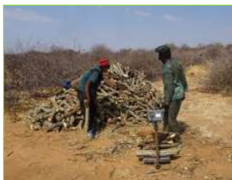
Picture 82: Wood load weighing for one traditional kiln at producer 1
