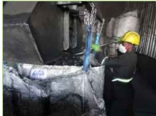
Picture 45: Charcoal sorting: sieve output (vibrating screen)
