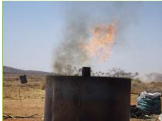
Picture 73: the gas going out the retort in flammable enough to burn
