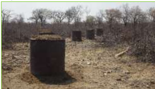
Picture 62: the kiln is sealed and let down to cool
