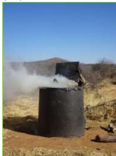
Picture 58: progressively the kiln is filled with wood on top of the fire
