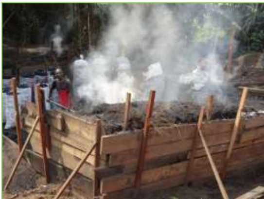
Picture 5: Traditional mound kiln in Cameroon (sawmill residues)
