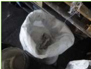
Picture 49: Starch is used as binder for briquette agglomeration
