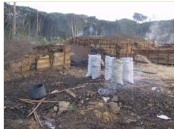
Picture 6: Traditional mound kiln in PR Congo (sawmill residues)
