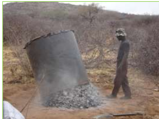
Picture 65: the charcoal produced contains burned wood & ashes
