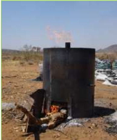
Picture 75: the retort needs to be fuelled permanently
